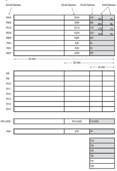
Fig 1: The programming model of the 8086 through the Core2 microprocessor including the 64-bit extensions.
