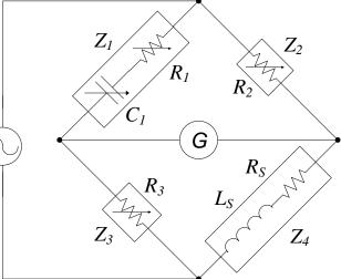
$$L_{S} = \frac{C_{1}R_{2}R_{3}}{1+w^{2}R_{1}^{2}C_{1}^{2}} = \frac{0.1n\times10k\times1k}{1+(3000)^{2}(20k)^{2}(0.1n)^{2}} = 1mH$$
