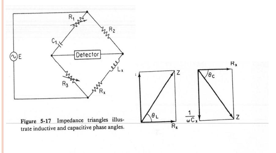
$$R_{x} = \frac{\omega^{2}C_{1}^{2}R_{1}R_{2}R_{3}}{1 + \omega^{2}C_{1}^{2}R_{1}^{2}}$$
